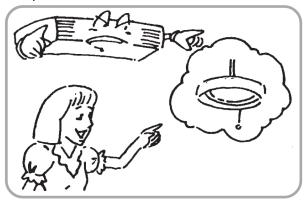
• Do not locate any obstacle against the air flow direction of indoor and outdoor unit. Inefficient performance or malfunction may result.
